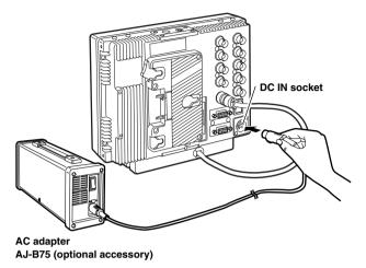
$2\,$  Set the power of the AC adapter to ON.
